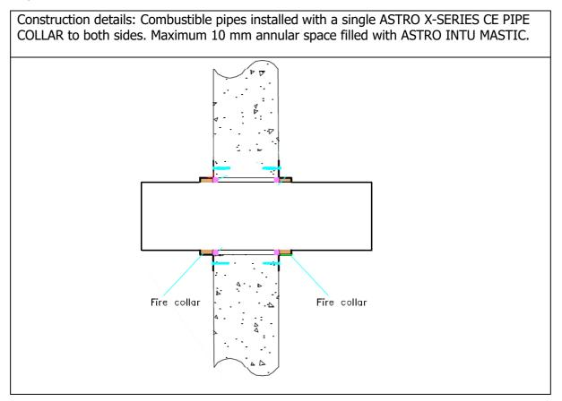
A.2.2.1 PP pipes with ASTRO X-SERIES CE PIPE COLLAR installed on both sides of rigid wall PP pipes according to EN 1451 with ASTRO X-SERIES CE PIPE COLLAR
