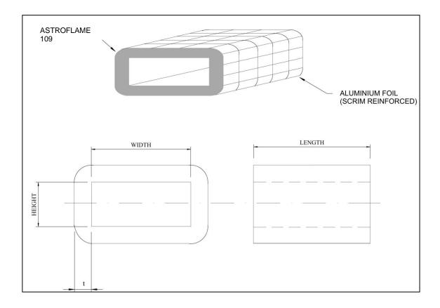
The Astro DS Duct Sleeve and Astro DS Duct Sleeve+ – Rectangular is available as single sleeve up to 500mm long which can be cut down to suit the intended application. It must be a minimum of 180mm long or longer if the supporting construction is thicker. The Astro DS Duct Sleeve and Astro DS Duct Sleeve+ is delivered in various sizes to fit particular duct sizes – see table below:
