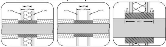
For timber stud partitions, seal must be  $\geq$ 100mm from studs with  $\geq$ 100mm of insulation (A1 or A2 to EN13501-1) between seal & stud. For further details check the ETA.
