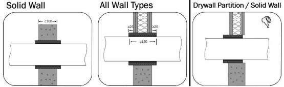
Rigid walls must comprise concrete, aerated concrete or masonry ≥650kg/m³ (Wall Type A) or concrete, masonry ≥1100kg/m³ (Wall Type B)
