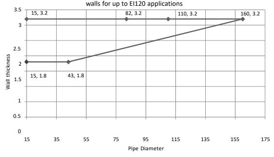
B.2.2 The line graphs below show the coverage of the allowable HDPE (according to EN 1519-1)\* pipe diameters and wall thickness for applications up to El120: (any pipe size variation along the lines and the area between the lines is covered)
