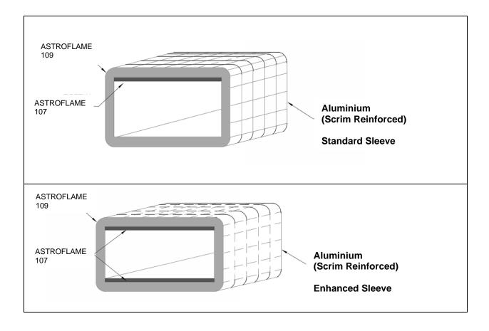
The Astro DS+ Low Profile (LP) Duct Sleeve – Rectangular is delivered in various sizes to fit particular duct sizes – see table below:
