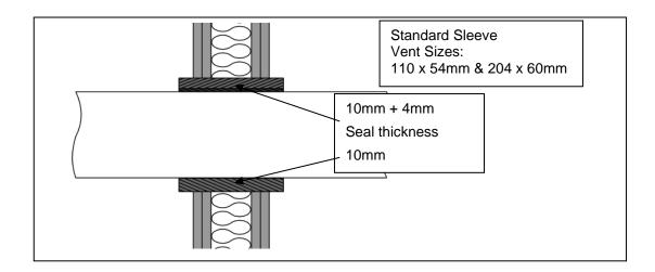
D.6 Field of application for Astro DS+ Low Profile (LP) Duct Sleeve – Rectangular (Enhanced Sleeve) for use with a 220mm wide x 90mm high PVC-U rectangular ambient pressure extraction and ventilation 'duct' type pipe penetrating fire resistant walls for applications up to El120:
