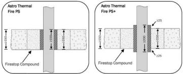
Rigid floors must comprise concrete ≥2400kg/m³ (Floor Type A) or ≥550kg/m³ (Floor Type B)
