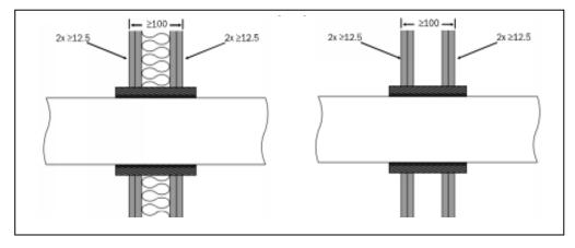
The seal must be a minimum of 250mm long with 75mm protruding each side
