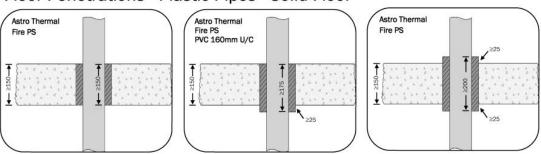
Rigid floors must comprise concrete ≥2400kg/m³ (Floor Type A) or ≥550kg/m³ (Floor Type B). For further details check the ETA
