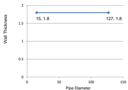
D.3 Field of application for minimum 250mm long Astro DS+ Low Profile (LP) Duct Sleeve – Circular (Enhanced Sleeve) for PVC-U circular ambient pressure extraction and ventilation 'duct' type pipes penetrating fire resistant walls for applications up to El120:
