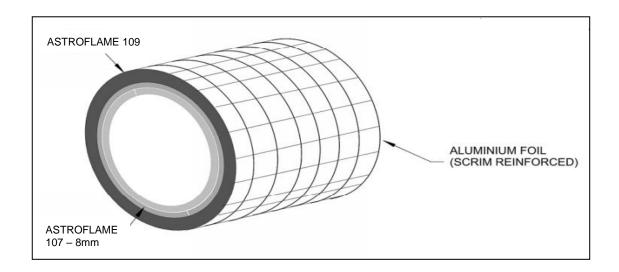
Astro Thermal Fire PS Fire Sleeve, Astro Thermal Fire PS+ Fire Sleeve and Astro DS+ Low Profile (LP) Duct Sleeve – Circular is available as single sleeve up to 500mm long which can be cut down to suit the intended application. It must be a minimum of 150mm long or longer if the wall is thicker. The Astro Thermal Fire PS Fire Sleeve, Astro Thermal Fire PS+ Fire Sleeve and Astro DS+ Low Profile (LP) Duct Sleeve is delivered in various sizes to fit particular pipe/duct diameters – see table below:
