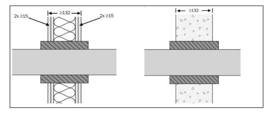
The seal must be a minimum of 180mm long with 24mm protruding each side of the wall
