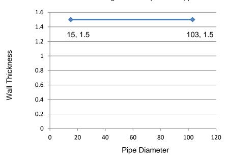
D.2 Field of application for minimum 250mm long Astro DS+ Low Profile (LP) Duct Sleeve – Circular (Standard Sleeve) for PVC-U circular ambient pressure extraction and ventilation 'duct' type pipes penetrating minimum 100mm thick fire resistant walls for applications up to El120:
