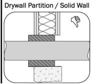
Rigid walls must comprise concrete, aerated concrete or masonry ≥650kg/m³ (Wall Type A) or concrete, masonry ≥1100kg/m³ (Wall Type B)
