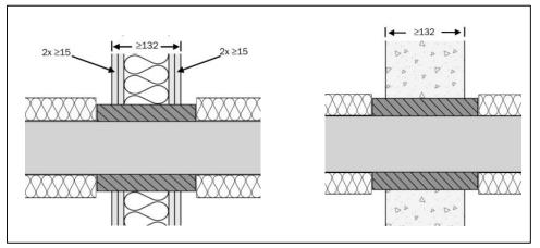
The seal must be a minimum of 150mm long with 9mm protruding each side of the wall
